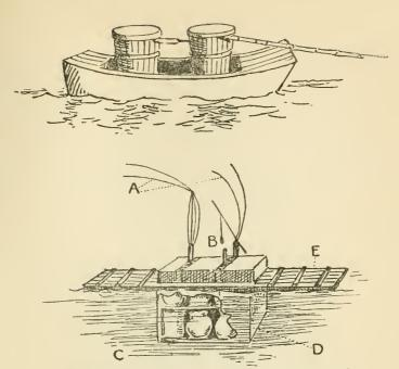
A, Wires to catch side of ship. B, Lead weight. C, Jars of Gunpowder. D, Case with side broken away to show jars. E, Raft.
